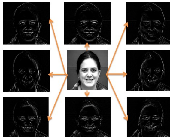
Figure.3 Edge responses of Prewitt operator in eight directions
