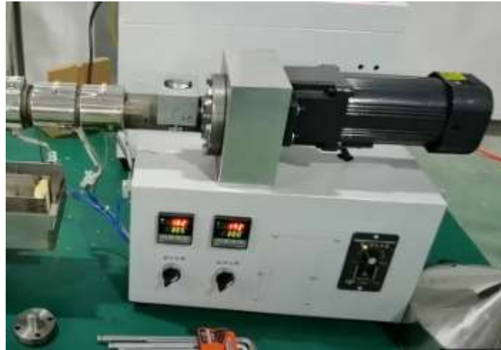
Figure 1: Extrusion machine sample used in the specimen preparation process
