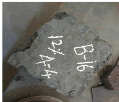
Fig. 5: Damaged edges at the periphery of specimen
